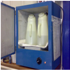
Resin heating oven
